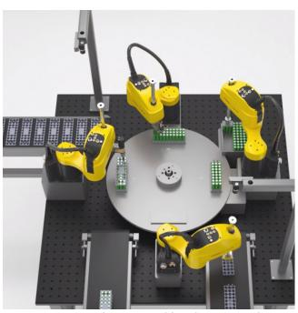
SR-3iA SCARA Robots assembling battery packs
